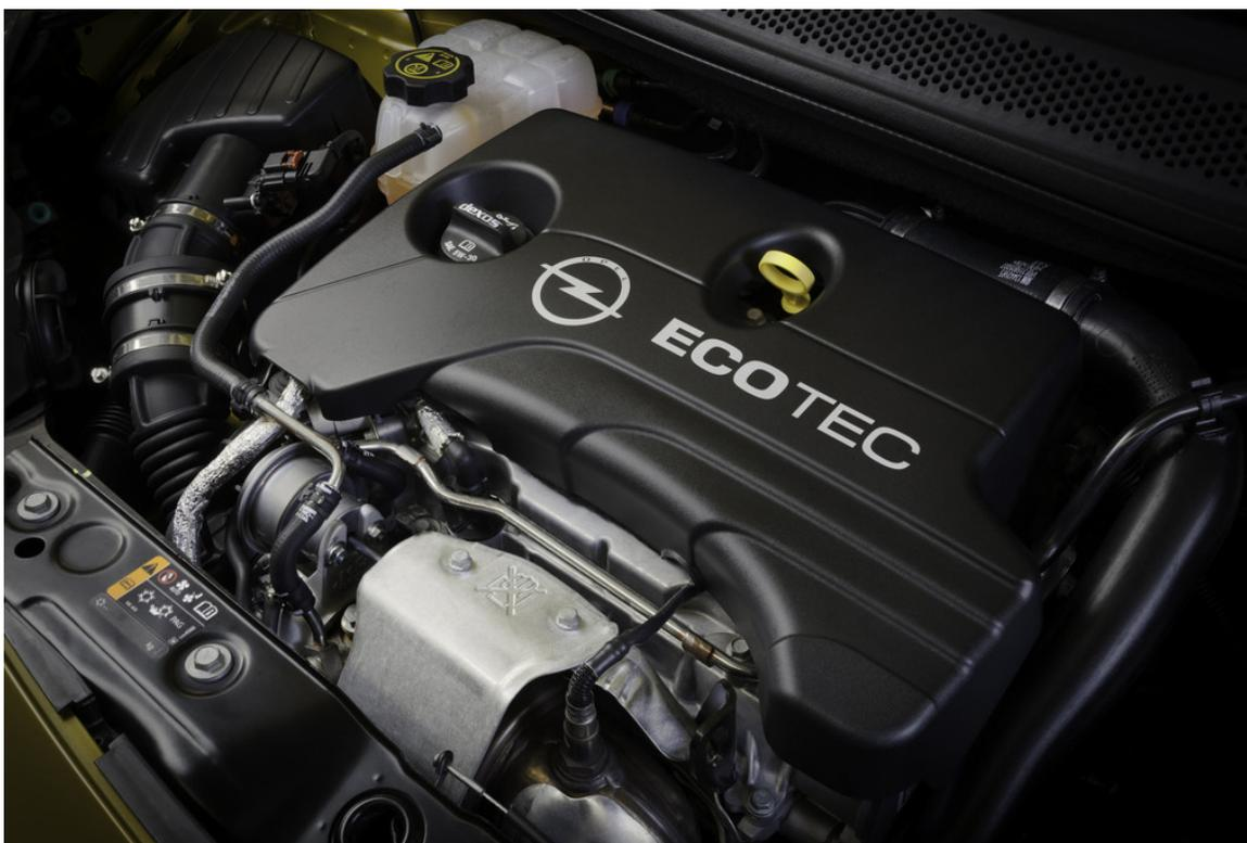
1.0 Ecotec Direct Injection Turbo von Opel.
